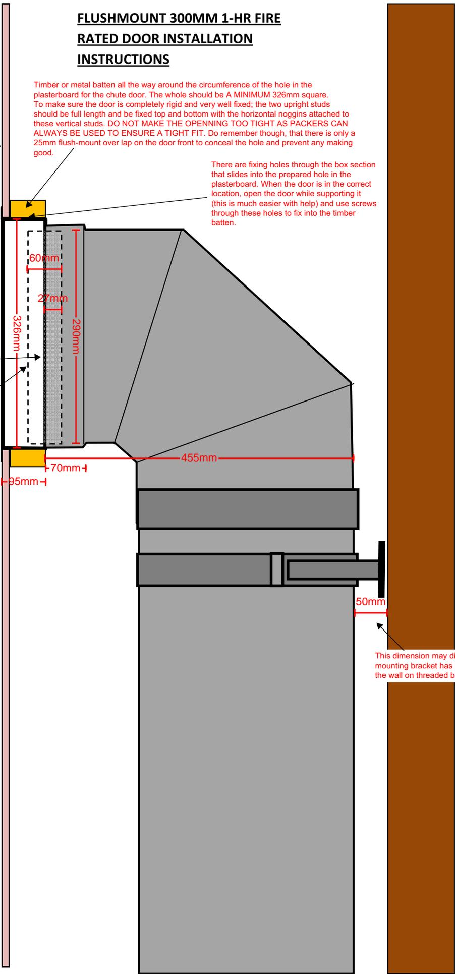
Diagram showing recommended internal stud-work for mounting of door.
