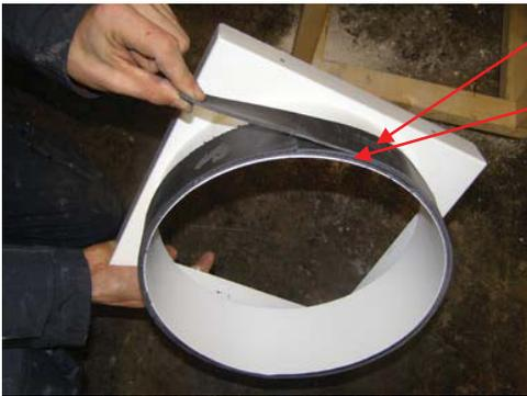
Attaching the sealing foam.
